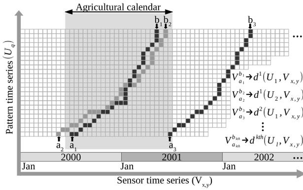
Fig. 4: Open boundary DTW alignment. Dark and light shades represent the alignments of the patterns  $U_1$  and  $U_2$ , respectively. The indexes  $a_k$  and  $b_k$  represent the starting and ending points of the  $k$ th alignment in  $\mathbf{V}$  associated with a DTW distance measure  $\delta_k$ .
