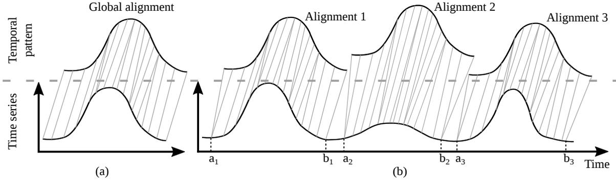
Fig. 2: (a) DTW Alignment between two time series with approximately same length, (b) DTW alignments between a pattern whose length is much shorter than the time series. The indexes  $a$  are starting points and  $b$  ending points of each interval in the long-term time series.
