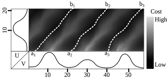
Fig. 3: Accumulated cost matrix  $D$  showing three possible alignment of the pattern  $U$  within the long-term time series  $V$ . The indexes  $a$  are starting points and  $b$  ending points of each DTW alignment in  $V$ .
